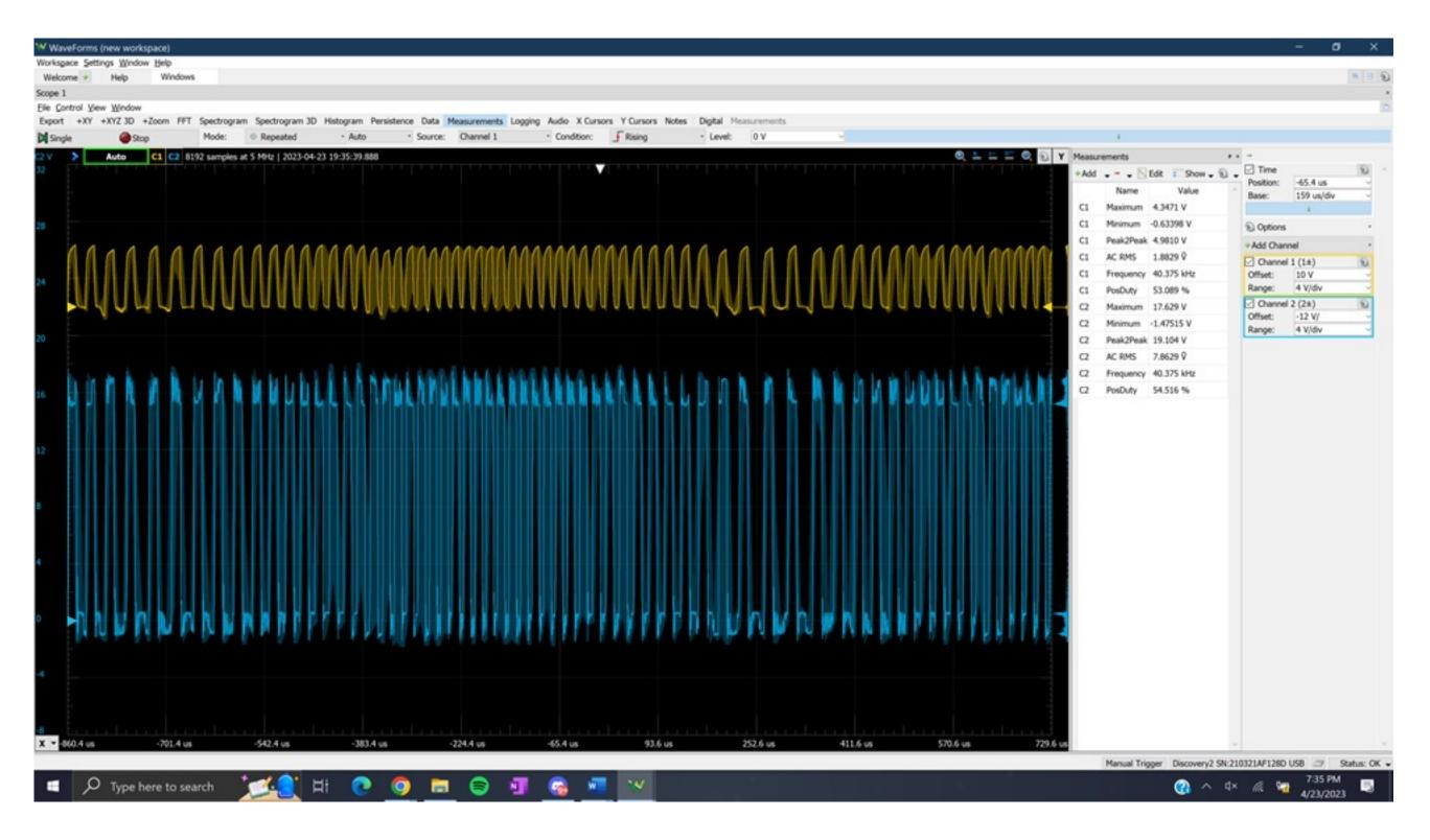
Next, the results of amplification are shown. The yellow plot measures a modulated signal going into the amplifier, and the blue plot measures the amplified signal. As can be seen in the vertical measurements shown, the amplifier produces a ~3.8x voltage increase in our configuration – enough to power the speakers.
