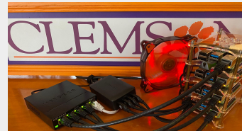
Figure 1: A Student's cluster, made from Raspberry Pi's
